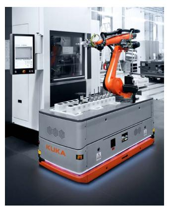
Next level: Tool automation thanks to mobile robotics. From price increases to shortages of skilled labor, industrial companies are under increasing pressure to meet demands for quality, volume and speed. In a pilot project, KUKA and HELLER, a producer of CNC machine tools, have developed a solution to these challenges: A KUKA KMR CYBERTECH automatically loads and unloads machines with tools and provides relief to employees.
