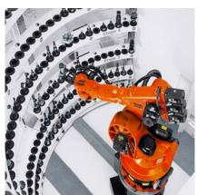
Tool change. In the case of large-scale tool magazines, robots support the handling of tools, e.g. in the "Tool Arena" of KUKA system partner Demmeler. This means there are no limits to your productivity even where 400 tools or more are required.
