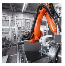
**Precision finishing.** Once set up, the robot performs tasks such as drilling or deburring reliably and with the utmost quality – and effectively interruption-free with an MTBF of 40,000 hours.
