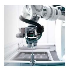
**Measuring.** Integrated measuring stations in the automation cell provide almost instantaneous information about the machining quality.
