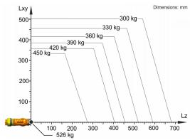
The KR 420 R3080 F is designed for a rated payload of 420 kg in order to optimize the dynamic performance of the robot. The maximum payload of 526 kg applies only if the position of the center of mass is 0 mm and a supplementary load optimized for the load case is mounted. The specific load case must be verified using KUKA.Load or KUKA Compose. For further consultation, please contact KUKA Support.
