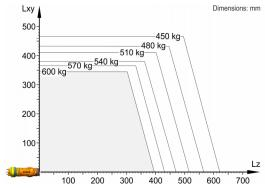
The KR 600 R2830 F is designed for a rated payload of 600 kg in order to optimize the dynamic performance of the robot. The maximum payload of 729 kg applies only if the position of the center of mass is 0 mm and a supplementary load optimized for the load case is mounted. The specific load case must be verified using KUKA.Load or KUKA Compose. For further consultation, please contact KUKA Support.
