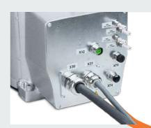
Integrated media supply for air, power and data. For minimum disruptive contours and maximum reliability in operation.
