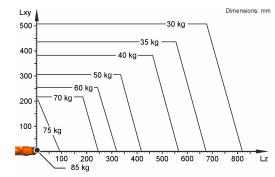
The KR 70 R2100 is designed for a rated payload of 70 kg in order to optimize the dynamic performance of the robot. With reduced load center distances and favorable supplementary loads, a maximum payload of up to 85 kg can be mounted. The specific KUKA Load case must be verified using KUKA. For further consultation, please contact KUKA Service.
