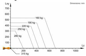
The KR 250 R2700-2 F is designed for a rated payload of 250 kg in order to optimize the dynamic performance of the robot. The maximum payload of 315 kg applies only if the position of the center of mass is 0 mm and a supplementary load optimized for the load case is mounted. The specific load case must be verified using KUKA.Load or KUKA Compose. For further consultation, please contact KUKA Support.
