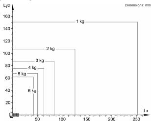
The KR 6 R500 Z200 is designed for a rated payload of 3 kg in order to optimize the dynamic performance of the manipulator. With the reduced load center distances, higher loads up to the maximum payload may be used. The specific load case must be verified using KUKA.Load. For further consultation, please contact KUKA Support.
