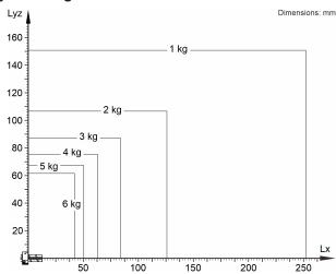
The KR 6 R500 Z200-2 is designed for a rated payload of 3 kg in order to optimize the dynamic performance of the manipulator. With the reduced load center distances, higher loads up to the maximum payload may be used. The specific load case must be verified using KUKA.Load. For further consultation, please contact KUKA Support.
