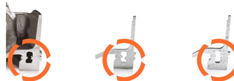
Reduction of the welding flash with optimized parameters (from left to right)
