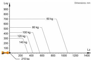
The KR 120 R3100-2 F is designed for a rated payload of 120 kg in order to optimize the dynamic performance of the robot. The maximum payload of 210 kg applies only if the position of the center of mass is 0 mm and a supplementary load optimized for the load case is mounted. The specific load case must be verified using KUKA.Load or KUKA Compose. For further consultation, please contact KUKA Support.
