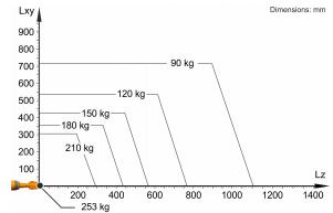
The KR 180 R2900-2 F is designed for a rated payload of 180 kg in order to optimize the dynamic performance of the robot. The maximum payload of 253 kg applies only if the position of the center of mass is 0 mm and a supplementary load optimized for the load case is mounted. The specific load case must be verified using KUKA.Load or KUKA Compose. For further consultation, please contact KUKA Support.
