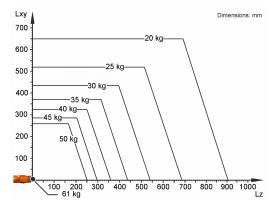
The KR 50 R2100 HO is designed for a rated payload of 50 kg in order to optimize the dynamic performance of the robot. With reduced load center distances and favorable supplementary loads, a maximum payload of up to 61 kg can be mounted. The specific KUKA Load case must be verified using KUKA. For further consultation, please contact KUKA Service.
