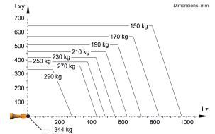
The KR 270 R3100-2 K is designed for a rated payload of 270 kg in order to optimize the dynamic performance of the robot. The maximum payload of 344 kg applies only if the position of the center of mass is 0 mm and a supplementary load optimized for the load case is mounted. The specific load case must be verified using KUKA.Load or KUKA Compose. For further consultation, please contact KUKA Support.
