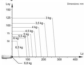
The KR 6 R700-2 is designed for a rated payload of 6 kg in order to optimize the dynamic performance of the robot. With reduced load center distances and favorable supplementary loads, a maximum payload of up to 6.8 kg can be mounted. The specific KUKA Load case must be verified using KUKA. For further consultation, please contact KUKA Service.
