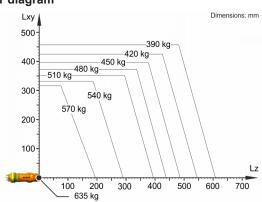
The KR 510 R3080 F is designed for a rated payload of 510 kg in order to optimize the dynamic performance of the robot. The maximum payload of 635 kg applies only if the position of the center of mass is 0 mm and a supplementary load optimized for the load case is mounted. The specific load case must be verified using KUKA.Load or KUKA Compose. For further consultation, please contact KUKA Support.
