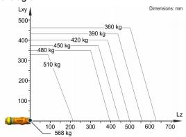
The KR 480 R3330 MT-F is designed for a rated payload of 480 kg in order to optimize the dynamic performance of the robot. The maximum payload of 568 kg applies only if the position of the center of mass is 0 mm and a supplementary load optimized for the load case is mounted. The specific load case must be verified using KUKA.Load or KUKA Compose. For further consultation, please contact KUKA Support.
