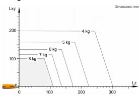
The KR 8 R1620 is designed for a rated payload of 8 kg in order to optimize the dynamic performance of the robot. With reduced load center distances, higher loads up to the maximum payload may be used. The specific load case must be verified using KUKA.Load. For further consultation, please contact KUKA Support.
