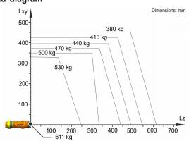
The KR 500 R2830 C-F is designed for a rated payload of 500 kg in order to optimize the dynamic performance of the robot. The maximum payload of 611 kg applies only if the position of the center of mass is 0 mm and a supplementary load optimized for the load case is mounted. The specific load case must be verified using KUKA.Load or KUKA Compose. For further consultation, please contact KUKA Support.
