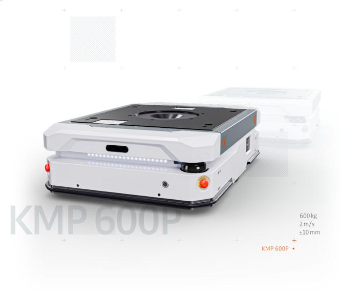
KMP 600 P The KMP 600P is a compact all-rounder that can transport up to 600 kilograms and is particularly suitable for cramped production environments. The autonomous mobile robot (AMR) offers an excellent price/performance ratio and, thanks to inductive charging, enables 24/7 operation and extended battery life.
