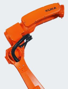
KR CYBERTECH nano ARC E. In the Edition variant, the KR CYBERTECH nano ARC E marks the entry into the world of welding automation. It has been created specifically for simple welding tasks. The KR CYBERTECH nano ARC E enables very cost-effective implementation of robot-based automation for processes of low complexity. At the same time, it is uncompromising when it comes to quality, accessories or software.
