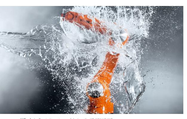
**WP robots.** Due to its waterproof design, the KR AGILUS WP is suitable for permanent use in working environments with splashing water. One example is the inside of machine tools. The WP robot meets the requirements of protection class IP 67 and is, therefore, even protected against temporary immersion in water. This is made possible by additional seals, constant surface treatment and the use of plastic covers instead of stainless steel covers.
