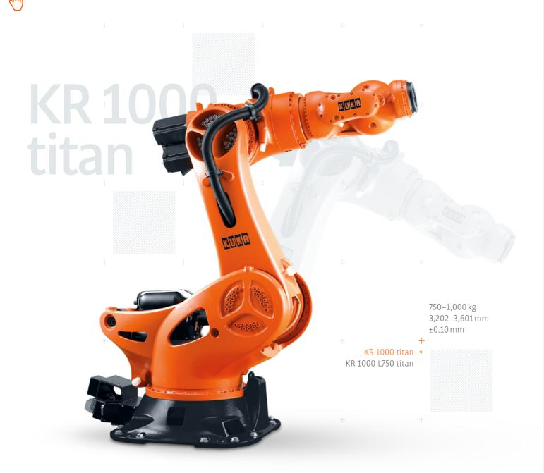
KR 1000 titan The heaviest workpieces and components even over long distances. The KR 1000 titan is our powerful robot for heavy loads and large, heavy tools with high mass inertias.
