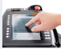
Efficient operator control with brilliant, capacitive touch display. Input the 8.4" screen.
