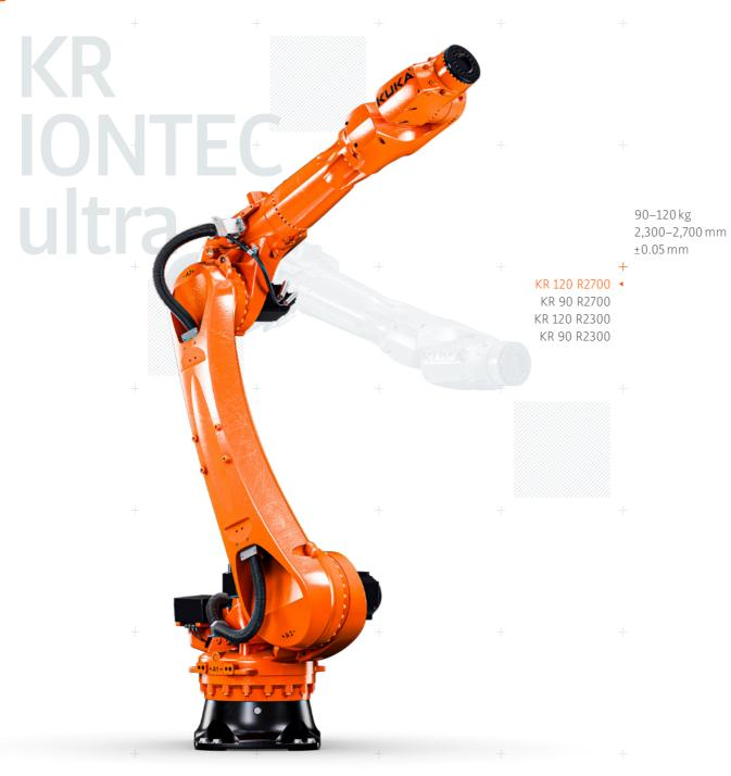
KR IONTEC ultra The KR IONTEC ultra is compact and powerful. With a payload range of 90 to 120 kilograms, the KR IONTEC ultra delivers top performance in confined spaces, making it is optimal for handling and welding applications.
