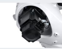
Additional brakes. Compared with the standard version of the KR QUANTEC series, additional brakes are integrated in axes 2 to 5. They ensure that the robot is stopped even if the first brake fails.
