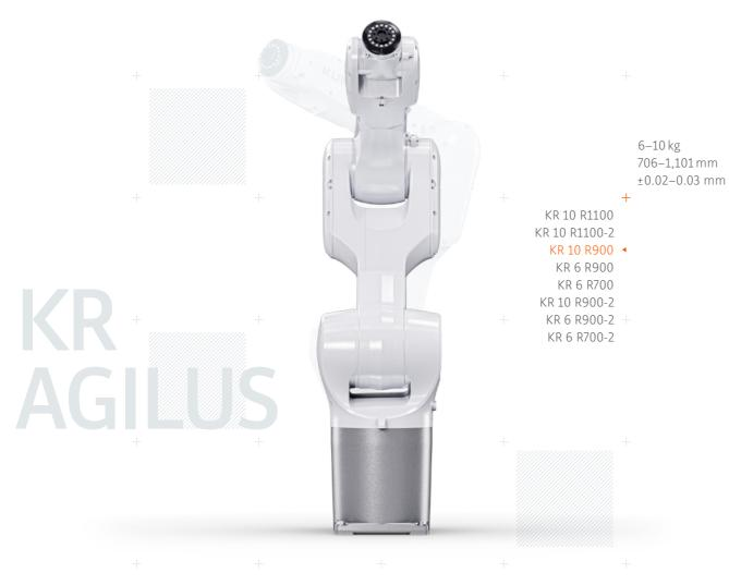
KR AGILUS The KR AGILUS sixx is our compact six-axis robot designed for particularly high working speeds. Different versions, installation positions, reaches and payloads transform the small robot into a precision artist.
