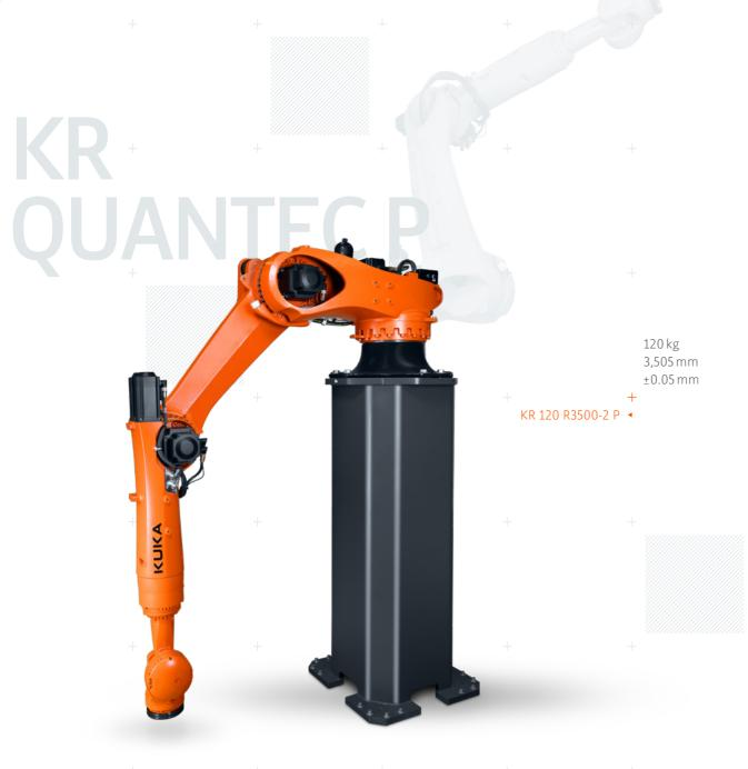
KR QUANTEC P The KR QUANTEC P is the KUKA industrial robot specially designed for press linking and is the first choice for loading, unloading and linking press lines.
