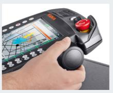
Simple robot jogging with the ergonomic 6D mouse. It offers intuitive jogging and reorientation of the robot in can be made quickly and easily via three or six degrees of freedom.
