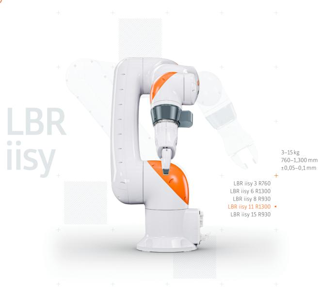
LBR iisy Flexible, intuitive to use, fast to implement and safe in direct contact with human colleagues – the LBR iisy is an all-around cobot for automated production. It combines the know-how, precision and reliability of industrial automation with the intuitive flexibility of a smart device.
