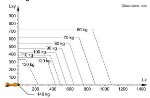
The KR 120 R3900-2 K is designed for a rated payload of 120 kg in order to optimize the dynamic performance of the robot. The maximum payload of 146 kg applies only if the position of the center of mass is 0 mm and a supplementary load optimized for the load case is mounted. The specific load case must be verified using KUKA.Load or KUKA Compose. For further consultation, please contact KUKA Support.
