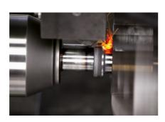
Removal of friction welding flash
