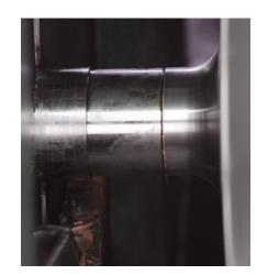
**01 Initial phase**Both workpieces are firmly clamped into the machine; one workpiece is rotated.
