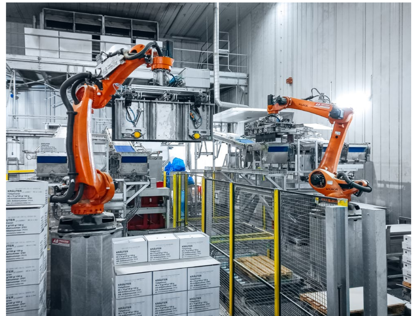
Under Arctic conditions at -25 °C, two KR QUANTEC PA Arctic robots palletize frozen aromatic herbs.
