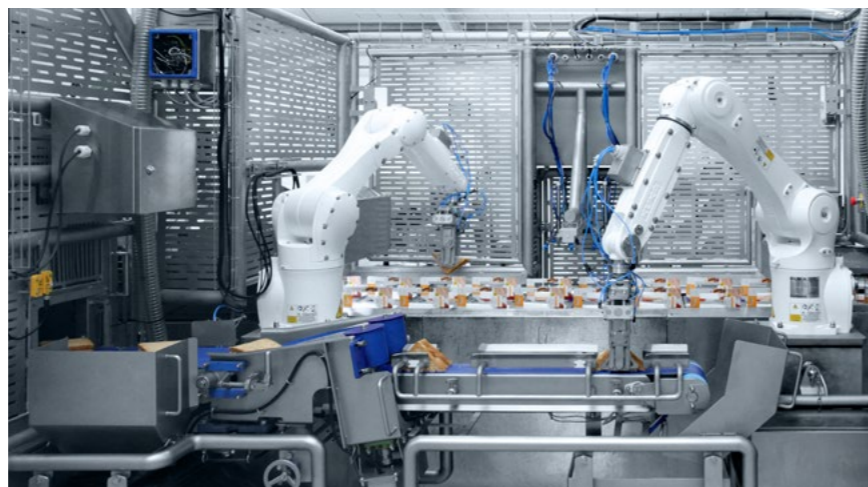
Hygienic, precise and cost-effective. Two KR AGILUS robots pack sandwiches.
