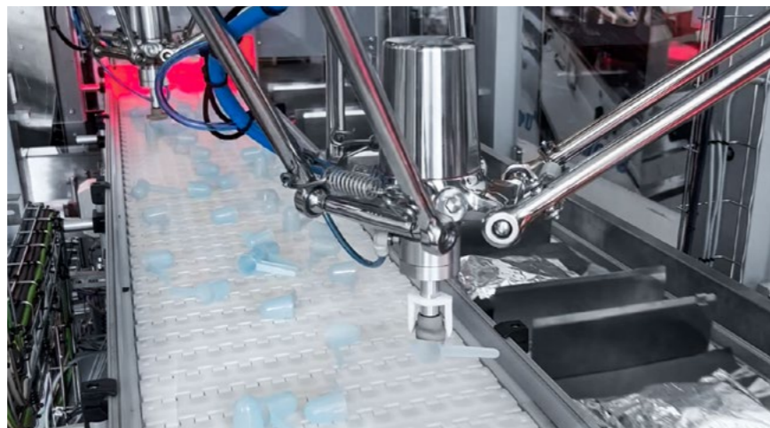
The KR DELTA places the spoons next to the bag with the baby food. In the next process step, both parts are placed in the packaging.
