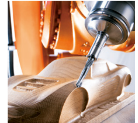
Direct execution of all standard G and M commands for tool handling and HSC (High-Speed Cutting).
