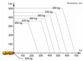
The KR 420 R3080 is designed for a rated payload of 420 kg in order to optimize the dynamic performance of the robot. The maximum payload of 526 kg applies only if the position of the center of mass is 0 mm and a supplementary load optimized for the load case is mounted. The specific load case must be verified using KUKA.Load or KUKA Compose. For further consultation, please contact KUKA Support.
