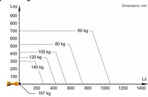
The KR 120 R2700-2 F is designed for a rated payload of 120 kg in order to optimize the dynamic performance of the robot. The maximum payload of 167 kg applies only if the position of the center of mass is 0 mm and a supplementary load optimized for the load case is mounted. The specific load case must be verified using KUKA.Load or KUKA Compose. For further consultation, please contact KUKA Support.
