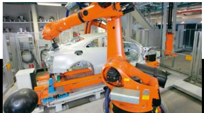
Welding, machining, removal of castings, or inline measurement of bodies-in-white: these are only a fraction of the possible applications.
